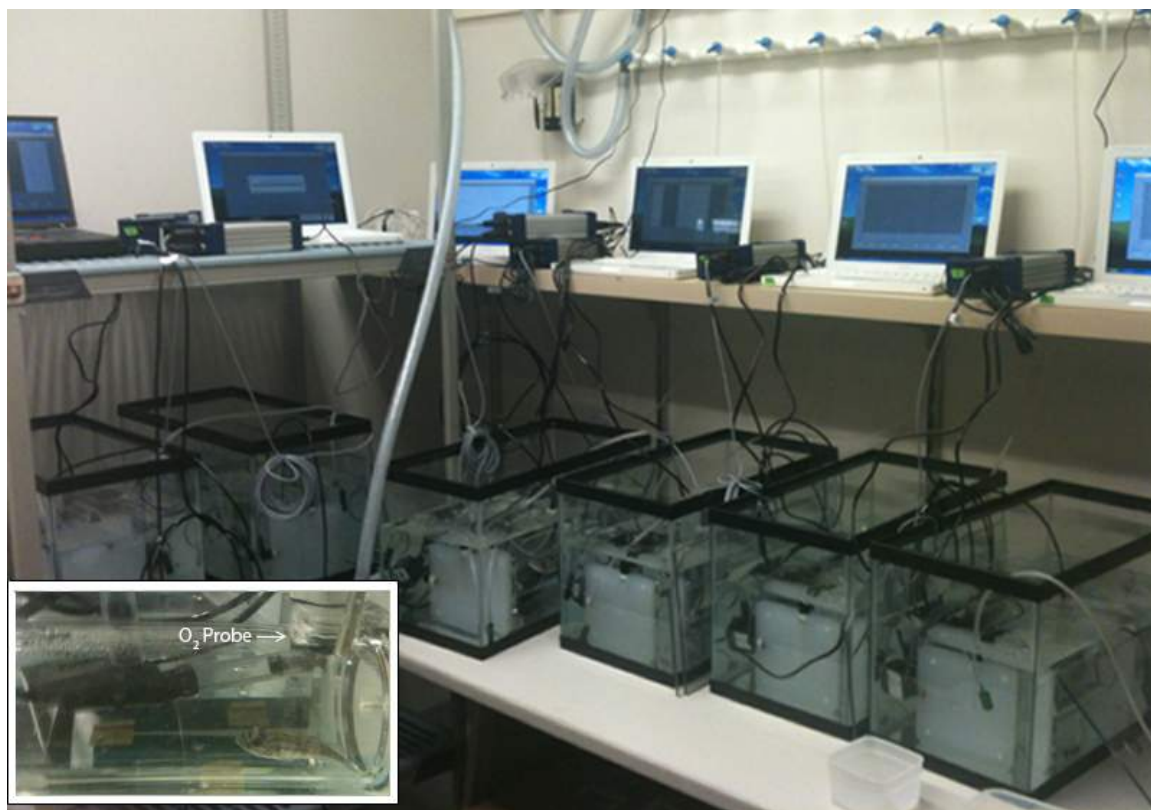
Figure 9. Respirometry set-up. The experimental workspace used in the present study. Originally, each cohort was to consist of six animals run in parallel; pump failure during the first session took one of the respirometers offline. The O 2 probe, thermometer, and water pumps were connected to each respirometer (blue/gray box beside each computer), which was itself connected to the computer. Figure inset in lower left corner depicts an animal inside the chamber; the location of the O 2 probe within the chamber is indicated in white text.
